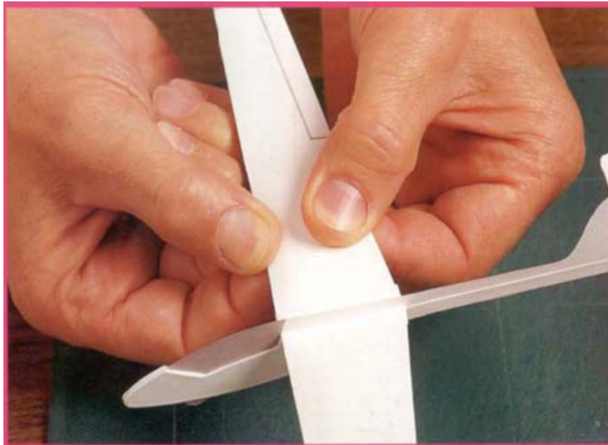
Figure 5 Adjusting Wing Curvature (Camber)
