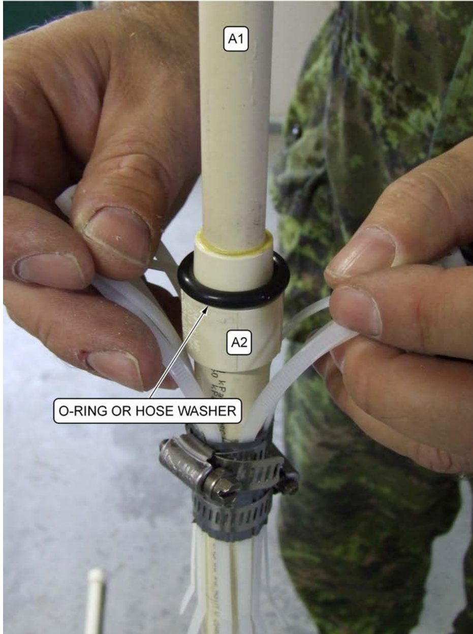
Figure A-23 Position of the O-Ring or Hose Washer on A2
