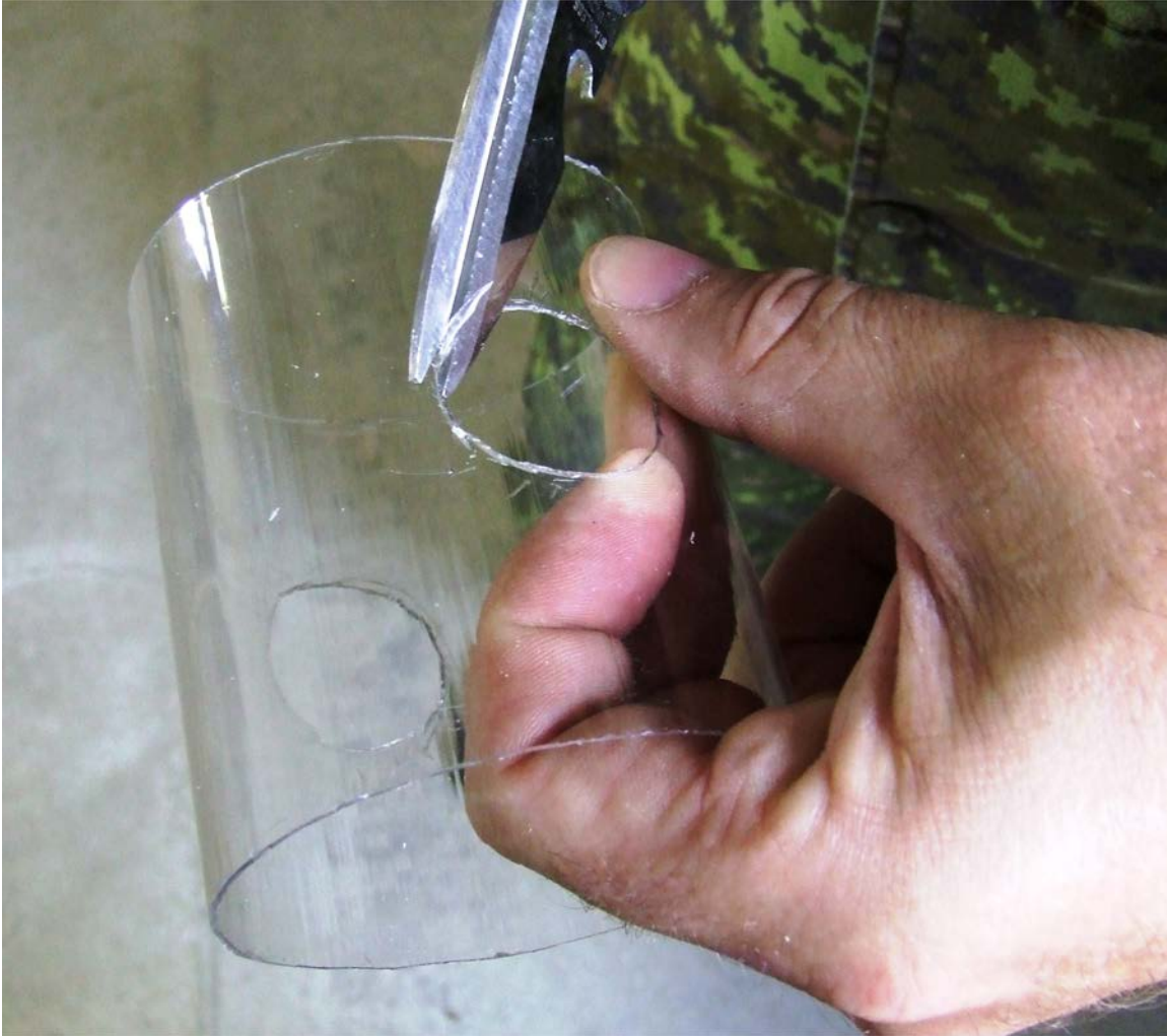
Figure A-27 Cutting the Hole in the Plastic Spring for Section A
