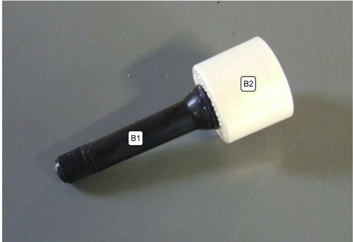
Figure A-12 Section B, Tire Valve Pulled Through B2
