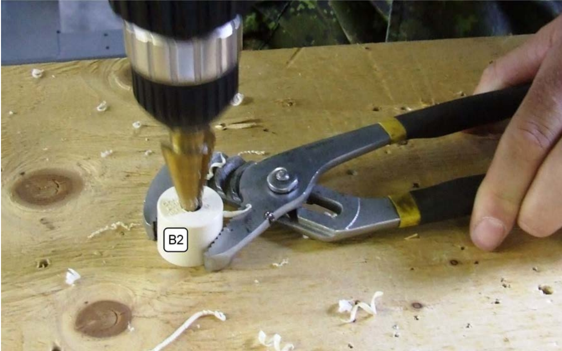
Figure A-11 Section B, Drilling the hole for the tire valve stem.
