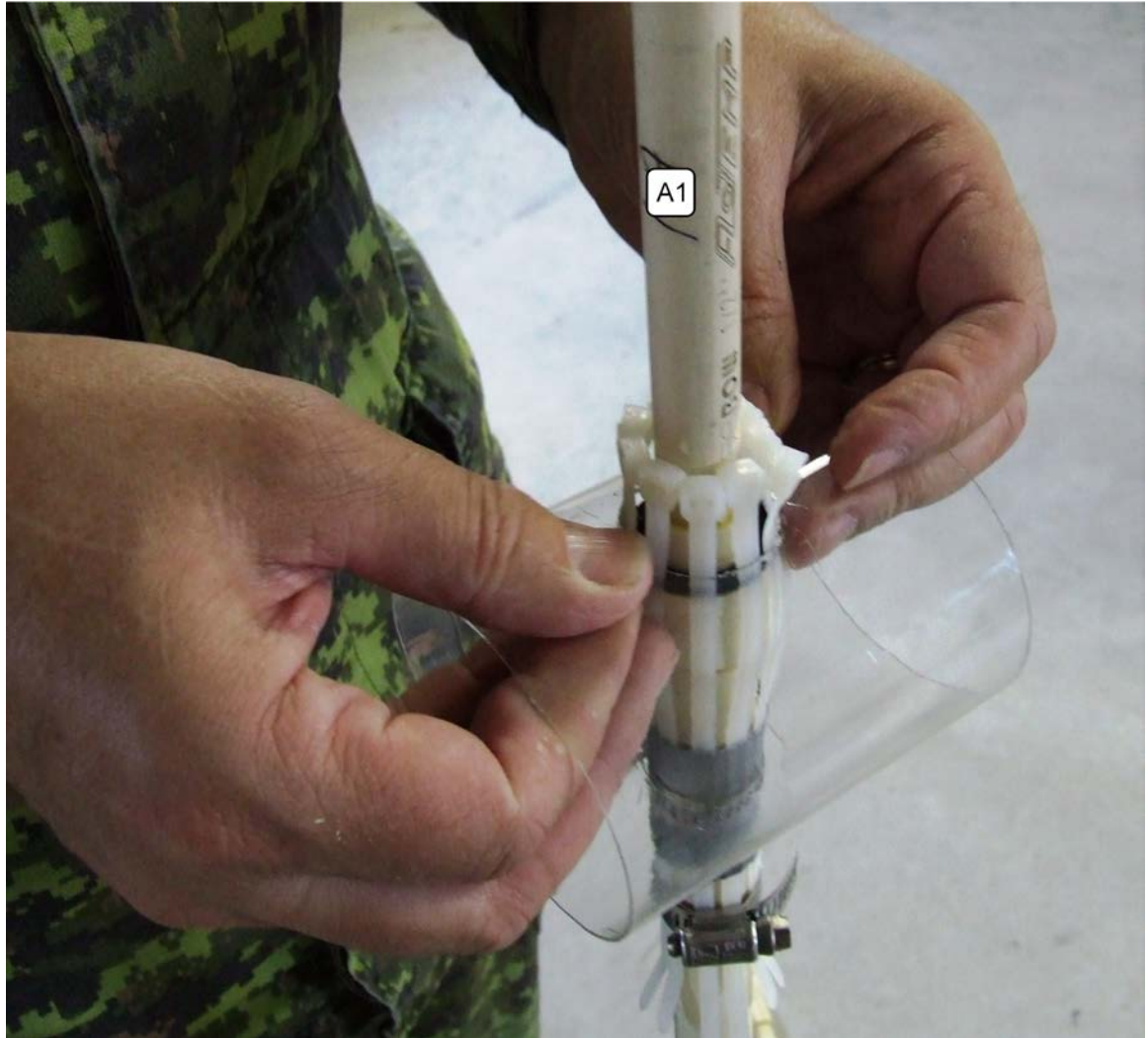
Figure A-28 Sliding the Spring over the Cable Ties
