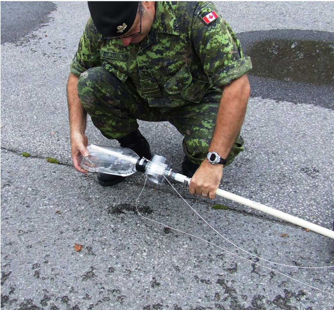
Figure A-31 Loading the Soda Bottle onto the Launch System
