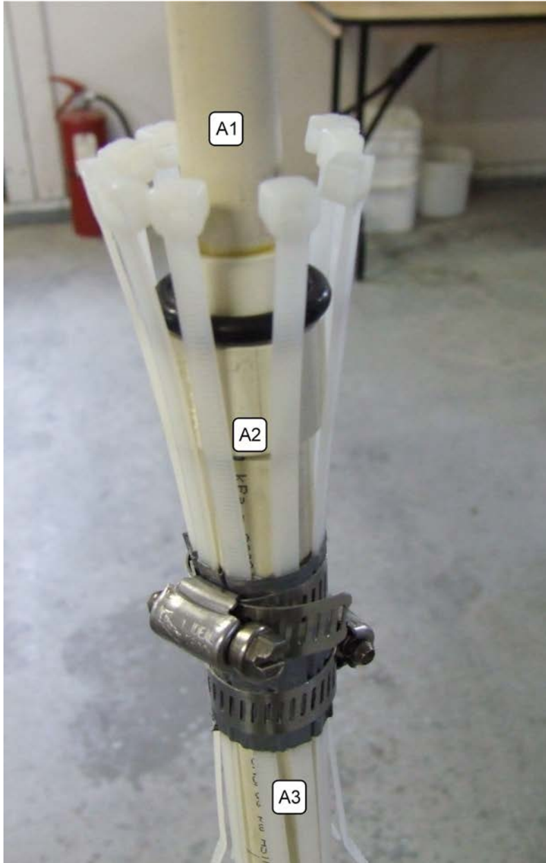
Figure A-25 Tie Cables Clamped to A3
