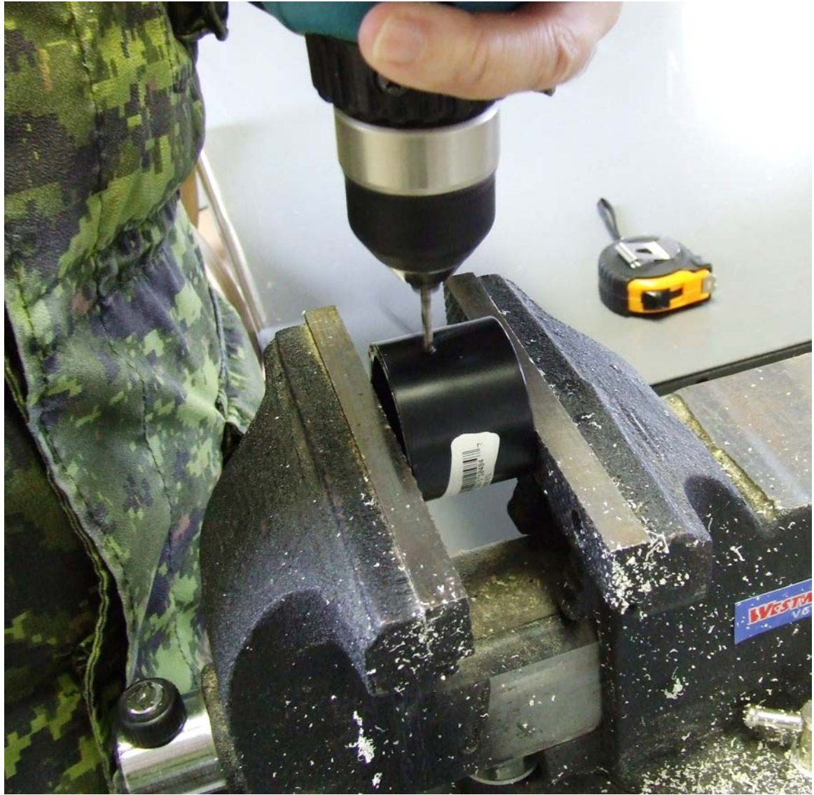
Figure A-26 Drilling 1/8-inch Holes in the ABS Coupler
