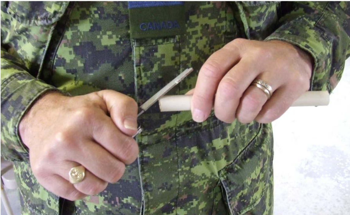
Figure A-5 Deburring the end of the tube with a hand file.
